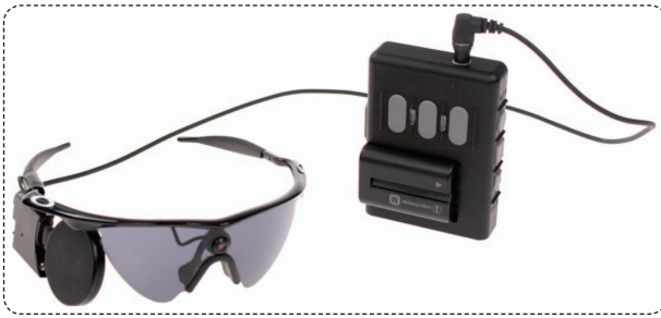
FIGURE 2 The external components of the Argus II include a pair of glasses with a very small video camera embedded in the bridge of the nose. The camera's video signal is processed by a rectangular, hip-worn computer (shown) called a VPU. The patient can control the signal for varying levels of contrast, brightness, and other parameters. (Photo courtesy of Second Sight Medical Products Inc.)
