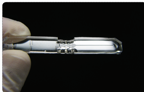
FIGURE 1 Rashid Bashir’s research group developed this device, which counts white blood cells from a whole-blood sample. It is made with polydimethylsiloxane (silicone), glass, and metal electrodes. (Photo courtesy of Rashid Bashir.)
