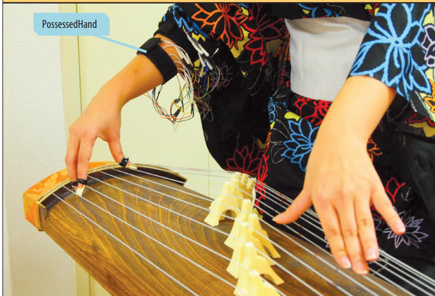
Figure 4. Using electrical stimulation, PossessedHand “tells” a beginning koto player which fingers to move and when, enabling the player to focus on the score’s string numbers.
