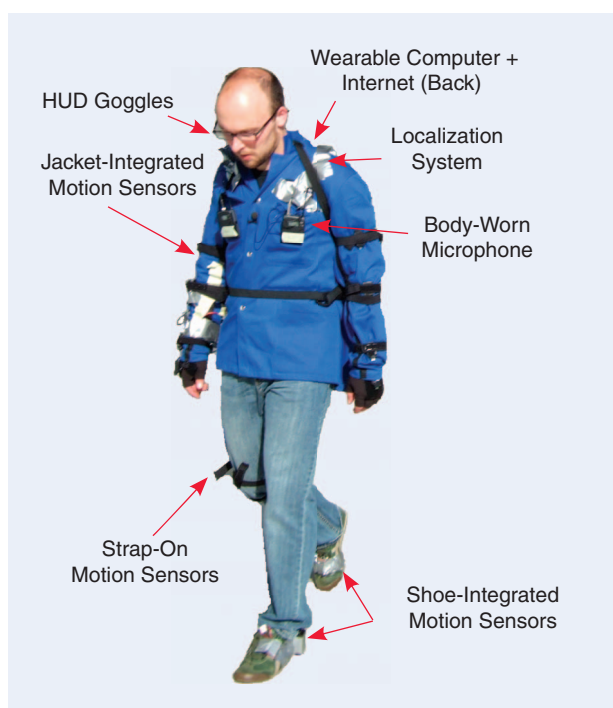
Figure 2. A typical wearable-computing system. The system comprises a see-through head-up display (HUD) in the goggles to provide the users with a contextual information, an Internet connection, an on-body computer, and sensors to infer the user's context, such as his activities and location.
