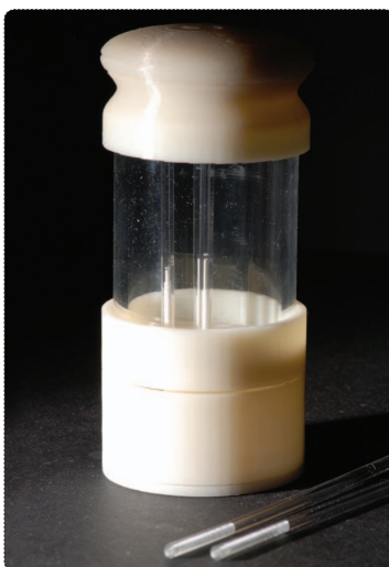
FIGURE 3 Rapid prototyping—SNAP—portable DNA isolation system.
